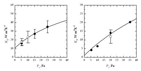
Fig. 3. Effect of chamber pressure on the value of  $K_v$  for the vial V<sub>1</sub> (left-side graph) and a stainless steel tray (right-side graph) processed in the laboratory freeze-dryer. The values calculated using the theoretical model, and the parameters of Table 3, are also displayed (solid line) together with the value estimated by pressure rise test technique ( $\Box$ )
