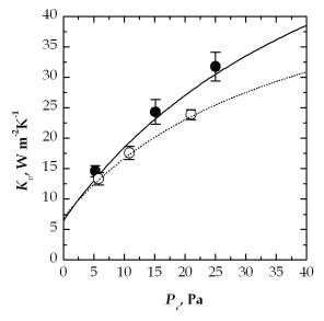
Fig. 8. Comparison between the value of  $K_v$  vs.  $P_c$  for vials subset E (processed in the laboratory freeze-dryer) in case of two different container geometries: ( $\bullet$ ) V<sub>1</sub> and ( $\bigcirc$ ) V<sub>2</sub> type. The values calculated using the theoretical model are also displayed: (solid line) vials V<sub>1</sub> and (dotted line) V<sub>2</sub>
