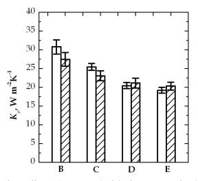
Fig. 10. Heat transfer coefficient (at  $P_c$ =10 Pa) of the four groups of vials (V<sub>2</sub> type, silane treated) in case of two different loading configurations: (void bars) the lot of vials is loaded on the heating shelf; (filled bar) the lot of vials is loaded on the heating shelf and enclosed by an external metal band
