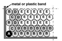
Fig. 1. Scheme of a lot, wherein vials have been classified depending on their position and on the additional heat transfer mechanisms involved
