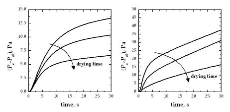
Fig. 2. Examples of pressure rise curves measured at various times during the primary drying stage in (left-side graph) a laboratory and (right-side graph) an industrial dryer
