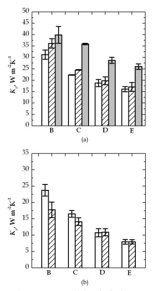
Fig. 12. Comparison between experimental values of  $K_v$  for the various groups of vials (V<sub>4</sub> type). (a) Influence of various loading configurations: vials loaded on a stainless steel tray ( $\Box$ ), a polystyrene tray ( $\blacksquare$ ) and directly on the heating shelf ( $\blacksquare$ ); (b) values measured in two pieces of equipment of different size: ( $\Box$ ) laboratory and ( $\boxtimes$ ) industrial scale dryer
