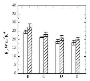
Fig. 9. Heat transfer coefficient of the four groups of vials (V<sub>2</sub> type) in case they underwent a silane coating treatment (void bars) or not (filled bar). The lot of vials is loaded on the heating shelf and enclosed by an external metal band. The measurement was carried out at  $P_c$ =10 Pa
