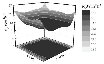
Fig. 4. Contour plot of the heat transfer coefficient for vials V<sub>1</sub> (loaded directly over the heating shelf) as measured over a lot. The primary drying phase was run at  $T_{\text{fluid}}$ =263 K and  $P_c$ =5 Pa. Results refer to a half of the batch
