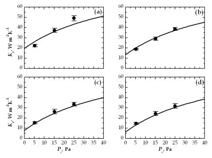
Fig. 6. Values of  $K_v$  vs.  $P_c$  for the four groups of vials (type V<sub>1</sub>) identified in Table 1: (a) vials B; (b) vials C; (c) vials D and (d) E
