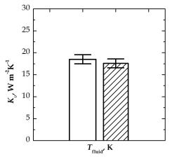
Fig. 5. Effect of  $T_{\text{fluid}}$ , and in turn of chamber gas temperature, on the value of  $K_v$  for the vial V<sub>2</sub> processed in the laboratory freeze-dryer. Both measurements were carried out at  $P_c$ =10 Pa, while the fluid temperature was set to: ( $\Box$ )  $T_{\text{fluid}}$ =275 K; ( $\boxtimes$ )  $T_{\text{fluid}}$ =253 K
