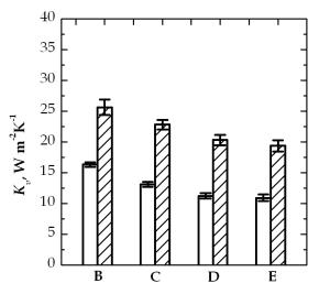
Fig. 11. Heat transfer coefficient (at  $P_c$ =10 Pa) of the four groups of vials (V<sub>3</sub> type) in case of two different loading configurations: (void bars) the lot of vials is loaded on a metal tray; (filled bar) the lot of vials is loaded on the heating shelf and enclosed by an external metal band
