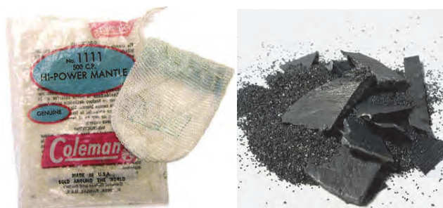
Fig. 1. Thorium dioxide with 1 percent cerium oxide impregnated fabric, Welsbach incandescent gas mantles (left) and ThO 2 flakes (right). Yttrium compounds now substitute for Th in mantles.
