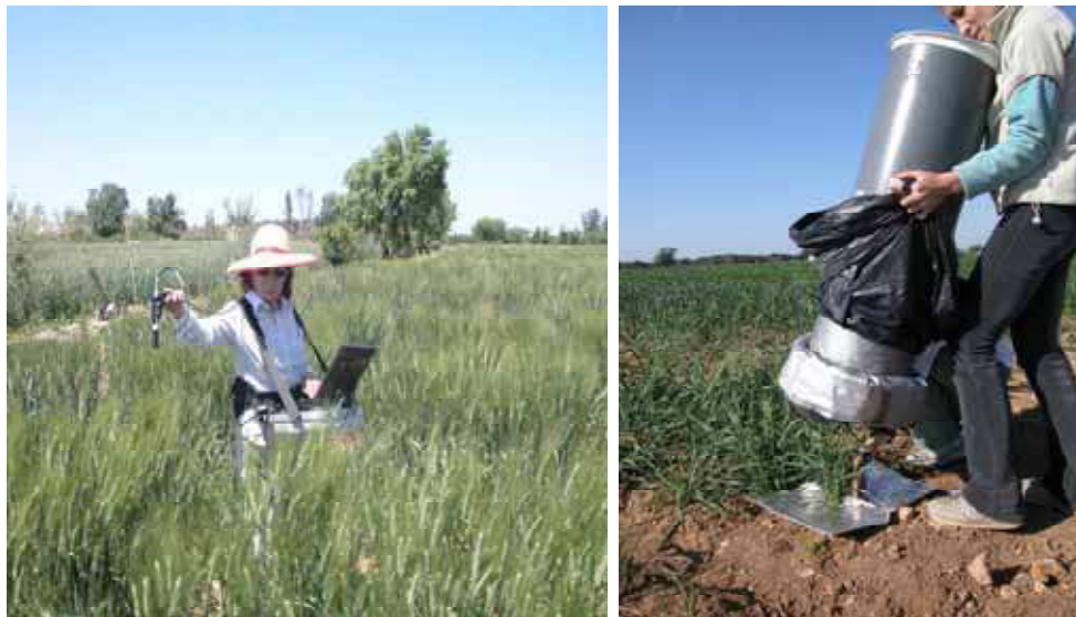
Fig. 5. Measurements of spectral reflectance on field plots and layout of the tube used by Álvaro et al. (2007) to capture the spectra of individual plants
