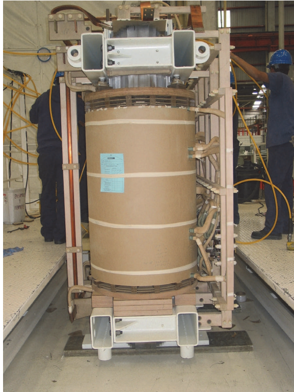
Fig. 2. Inner part of the transformer. The core and coils assembly is shown at the manufacturing stage. (Courtesy of Prolec GE ).
