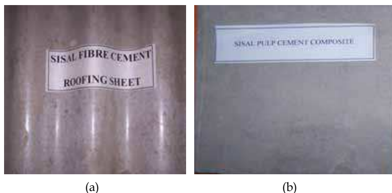
Fig. 7.3.1 Sisal composites: (a) Sisal fiber cement roofing sheet (b) Sisal pulp cement composites panel
