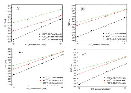
Fig. 6.  $CO_2$  concentration vs. EMF for the  $CO_2$  gas sensors attached with (a)  $Na_2CO_3$ - $CaCO_3$  = 1:0, (b)  $Na_2CO_3$ - $CaCO_3$  = 1:0.5, (c)  $Na_2CO_3$ - $CaCO_3$  = 1:1.5, and (d)  $Na_2CO_3$ - $CaCO_3$  = 1:2 [18].
