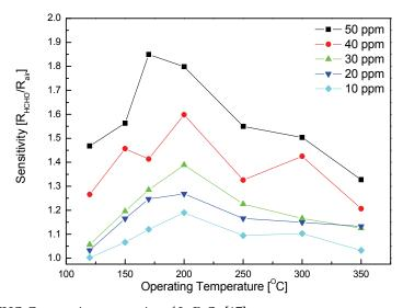
Fig. 7. HCHO Gas-sensing properties of LaFeO<sub>3</sub> [17].
