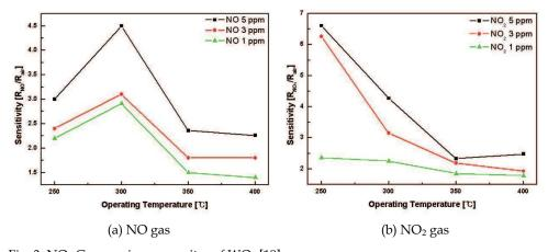
Fig. 3. NO<sub>x</sub> Gas-sensing properites of WO<sub>3</sub> [19].
