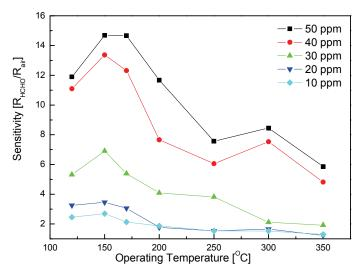
Fig. 8. HCHO Gas-sensing properties of La<sub>0.8</sub>Sr<sub>0.2</sub>FeO<sub>3</sub> [17].
