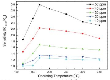
Fig. 9. HCHO Gas-sensing properties of La<sub>0.5</sub>Sr<sub>0.5</sub>FeO<sub>3</sub> [17].
