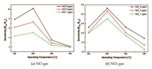
Fig. 4. NO<sub>x</sub> Gas-sensing properites of In<sub>2</sub>O<sub>3</sub> [19].
