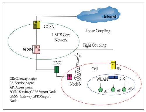
Fig. 1. Tight coupling and loose coupling
