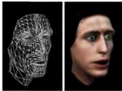
Figure 16. In the left panel is shown the mesh model of the talking head. In the right panel, a skin has been added to the model
