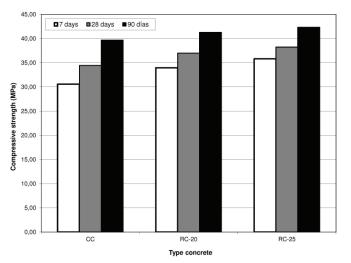
Fig. 2. Compressive strength of the concretes
