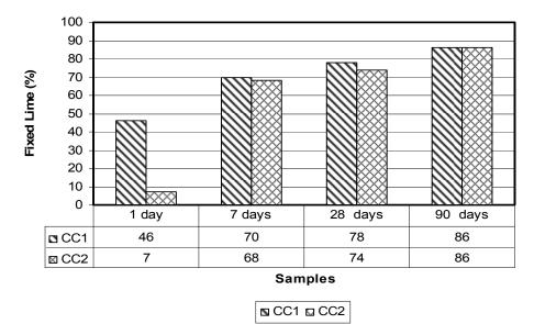
Fig. 6. Pozzolanic activity of the two types of ceramic rubble
