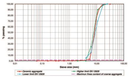
Fig. 1. Particle size grading of ceramic aggregate
