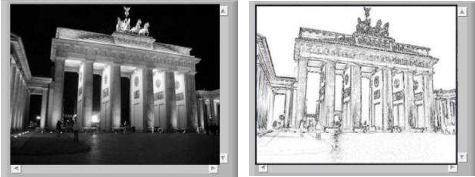
Fig. 11. Sobel Edge Detector. (a) Grayscale image, (b) Sobel Transformation.
