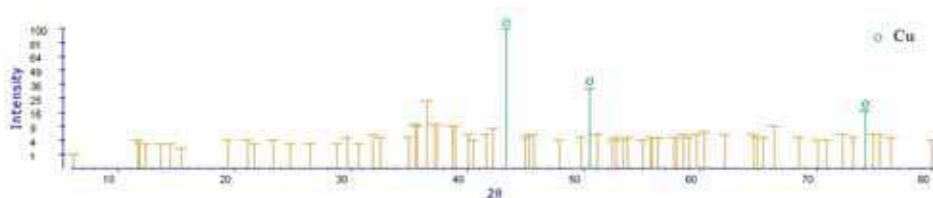
Fig. 8. XRD pattern of \text{Cu-2Al}_2\text{O}_3
