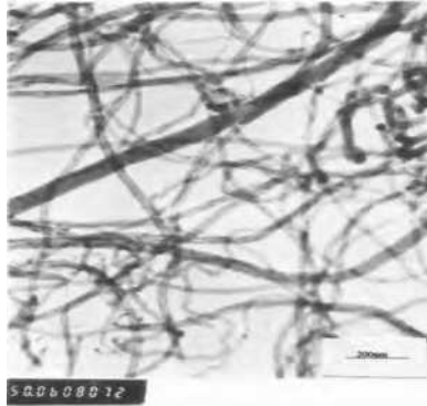
Fig. 3. TEM image of dispersed ACNTs
