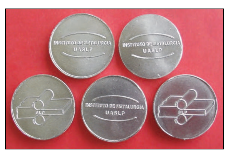
Fig. 14. Medals elaborated with aluminum clad zinalco.
