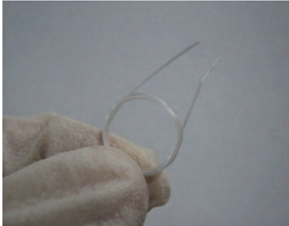
Fig. 5. Polymer based flexible piezoelectric fibre generated by a continuous process using the melt extruder.
