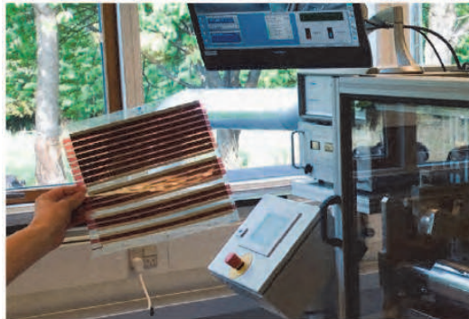
Fig. 12. Photograph of one of the final modules in front of the R2R coater. From Ref. (Krebs et al., 2009).
