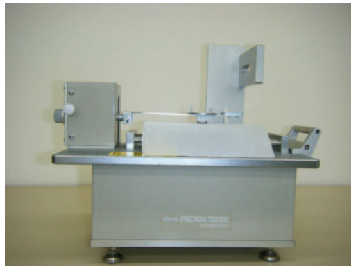
Fig. 2. KES-SE surface friction tester
