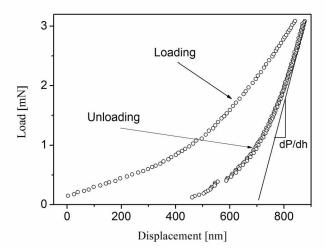
Fig. 2. Typical loading and unloading displacement curves during a nanoindentation cycle on AryLite $^{\text{TM}}$  substrate
