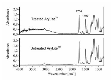
Fig. 4. ATR spectra of AryLite $^{\text{TM}}$  before and after surface silane treatment in the range 4000-700 cm $^{\text{-}1}$
