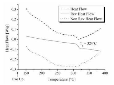
Fig. 3. Modulated Differential Scanning Calorimetry of AryLite™.
