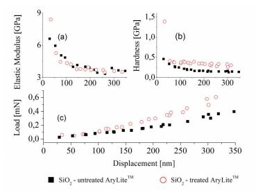
Fig. 6. Young's modulus (a), hardness (b) and load vs. depth (c) of untreated and treated AryLite<sup>TM</sup> coated with  $SiO_2$  layer
