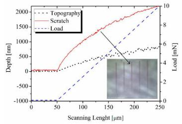
Fig. 8. Scratch test curve of  $SiO_2$  layer of treated AryLite<sup>TM</sup> with optical image in the plot inset (magnification 20x). Topography and scratch scan refers to the third wear
