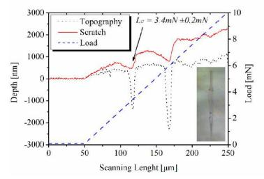
Fig. 7. Scratch test curve of  $SiO_2$  layer of untreated AryLite<sup>TM</sup> with optical image in the plot inset (magnification 20x)
