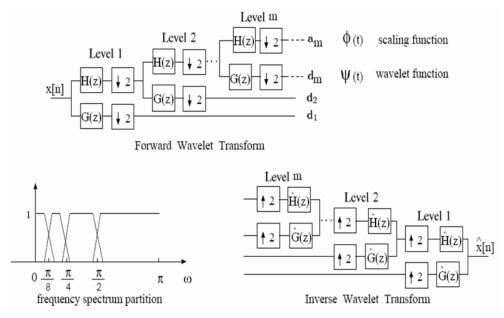
Fig. 4. The DWT implementation using a filter bank structure.
