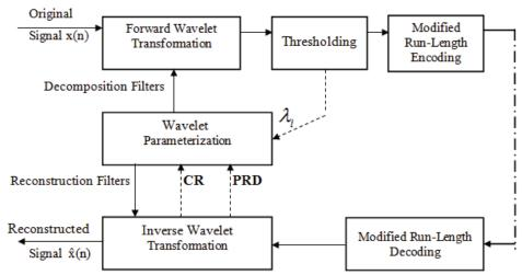
Fig. 6. Block diagram for the proposed compression algorithm.
