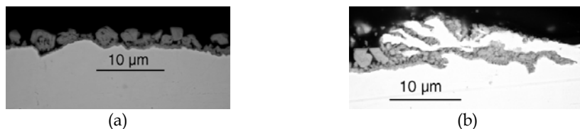
Fig. 27. Cross sections after cyclic corrosion test ( 1\text{A}\cdot\text{dm}^{-2} ) of the lead coating annealed at 80^\circ\text{C} (a), at 110^\circ\text{C} (b) (local infiltrations of corrosion products under the coating)
