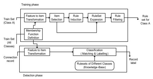
Fig. 5. Block diagram for IDS framework (Tajbakhsh et al., 2009)
