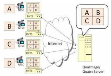
Fig. 5. Mechanism provided by QualImage/ Quatre system
