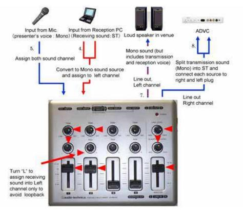
Fig. 4. Configuration diagram for setting audio
