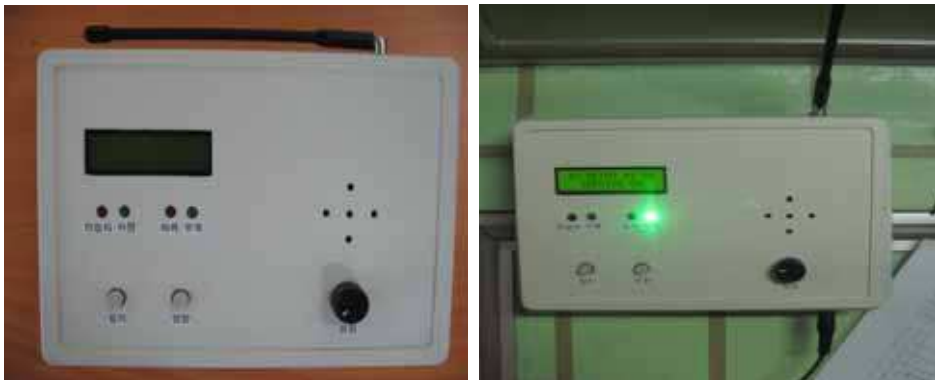
Fig. 10. Prototype of the motor-car terminal
