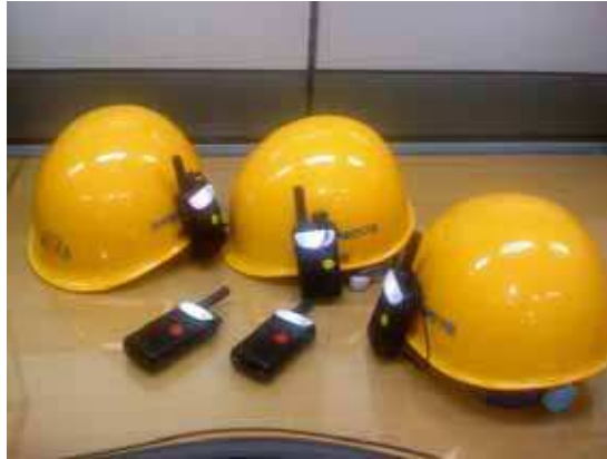
Fig. 17. Result of the prototype safety helmet for railways with bone conduction method
