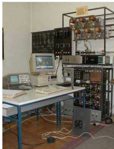
Fig. 10. CSI fed induction motor drive with improved vector control algorithm: control block diagram (left), laboratory prototype (right)
