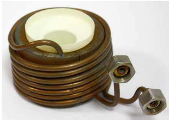
Fig. 8. Evaporator with inductor-concentrator equipped with crucible, which allows avoiding migration of liquid metal towards the outer crucible surface
