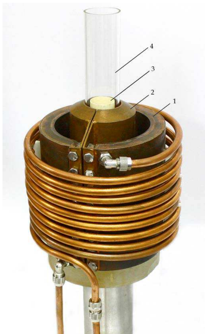
Fig. 17. Photograph of the induction evaporator for metallization of the inner surface of dielectric tubes. 1 is the secondary winding of the RF auto-type transformer, 2 is the working inductor for crucible heating, 3 is the heat shield for protection of substrate from overheating, 4 is the glass tube (substrate)
