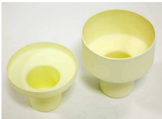
Fig. 5. Pyrolytic BN crucibles with outwardly directed funnel-shaped lips to avoid migration of liquid metal towards the outer crucible surface
