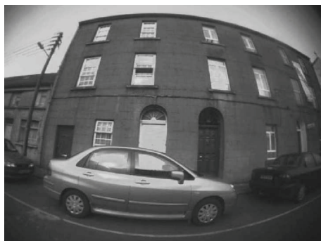
Fig. 6. Automotive fish-eye example illustrating the effects of fisheye distortion.
