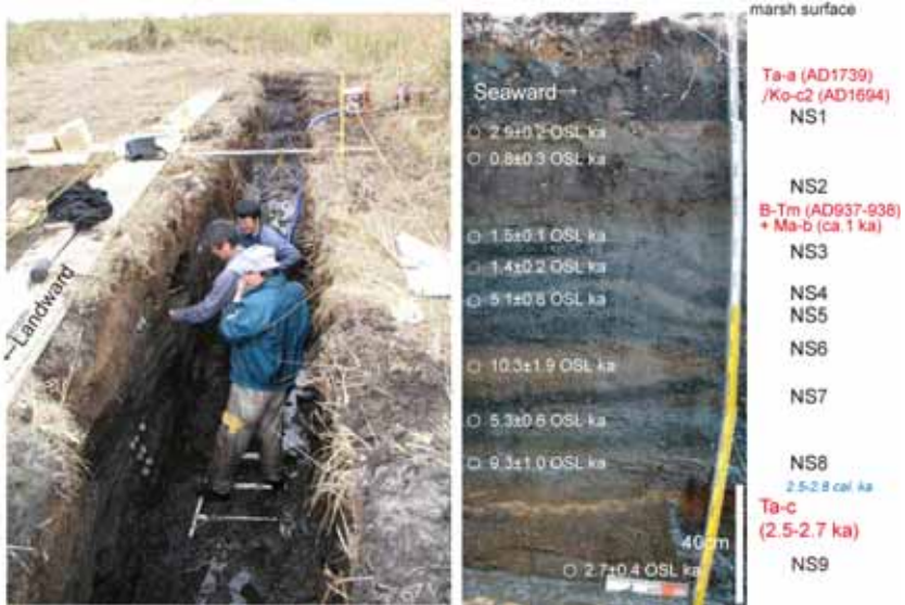
Fig. 6. Collection of samples for OSL dating at Shig trench (left). Photograph of the trench wall showing the OSL sampling horizons and dating results (right). AMS 14 C dating results, tephra layers and dates, and sand beds NS1 to NS9 are indicated to the right of the photograph.
