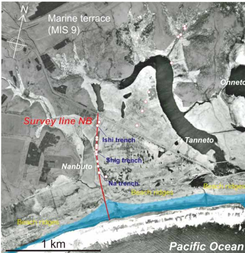
Fig. 2. Aerial photograph showing the topography around Nanbuto marsh, and the locations of three of the trenches excavated along survey line NB. Circles show sites where 17th century tsunami deposits (layer NS1) were observed. The blue shading shows the area inundated by the 1973 Nemuro-oki tsunami. Dark gray shading shows MIS 9 marine terrace surfaces, and light gray shading shows the area inundated by the 17th century tsunami (estimated from the distribution of NS1).
