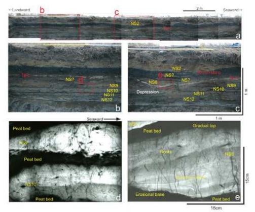
Fig. 4. Wall photographs of Ishi trench, the most inland trench (a); close-ups of portions of the wall (b, c); and radiographs of typical tsunami deposits (d, e) in this trench.
