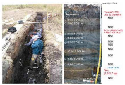
Fig. 6. Collection of samples for OSL dating at Shig trench (left). Photograph of the trench wall showing the OSL sampling horizons and dating results (right). AMS <sup>14</sup>C dating results, tephra layers and dates, and sand beds NS1 to NS9 are indicated to the right of the photograph.
