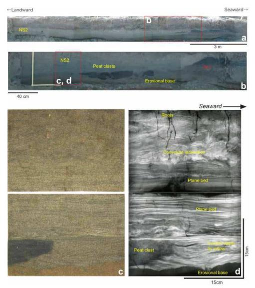
Fig. 5. Na trench, at the seaward location of the survey line, in Nanbuto marsh. Trench wall photographs (a, b); photograph of the oriented plastic-box sample of NS2; (c) radiograph of the same sample with sedimentary interpretation (d).
