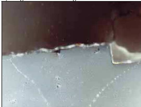
c) fatigue fracture contour
