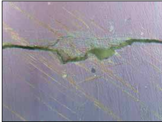
a) transcrystalline fatigue crack growth with the slip bands
