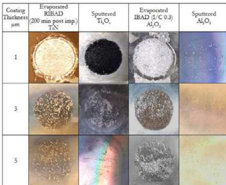
Fig. n.3.10. Showing extent of surface damage following immersion of the various coated substrate in acidified 5% NaCl solution at PH 6 and 20°C for 48 hours.
