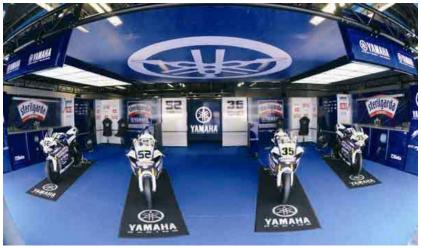
Fig. 10. New lighting system on the box Yamaha, with LED panel (Photo agency: Alex Photo) Specifically, the lighting system, showen in Fig. 10, was characterized by: 24 LED panels (Lumisheet, 21W, Fawoo) drawed to each other and arranged in two sections of the ceiling, 4 linear suspension elements LED (Linealuce, 37W, Maytag) and 4 LED projectors (Miniwoody, iGuzzini) as.
