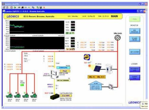
Fig. 20. Remote monitoring display
