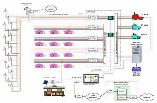
Fig. 11. Typical layout of the hybrid system
