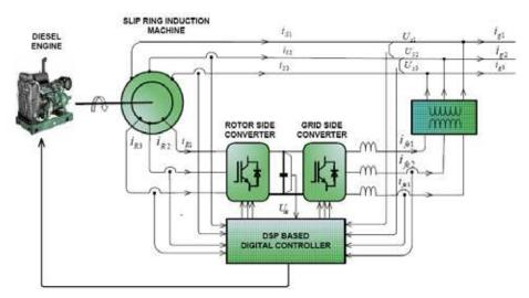
Fig. 26. Diesel powered Variable speed Doubly Fed Induction Generator
