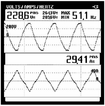
Fig. 9.a - Typical voltage and current waveforms
