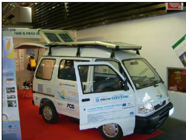
Fig. 10. A prototype of Hybrid Solar Vehicle with series structure developed at the University of Salerno.
