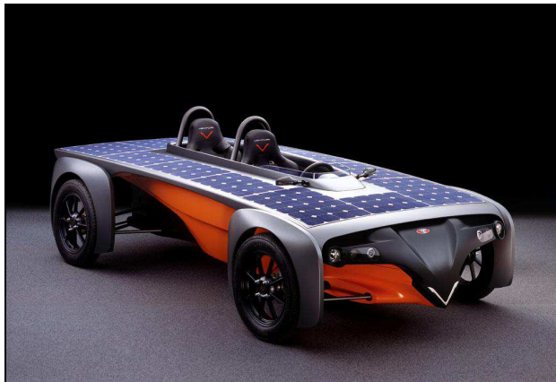
Fig. 3. Astrolab, a Hybrid Solar Vehicle developed by the French company Venturi.
