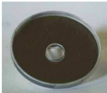
Fig. 5. Collector A1 (Mangin60) realized in glass.
