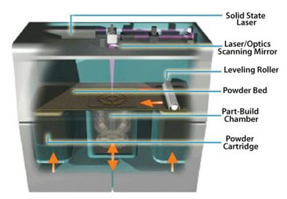
Fig. 3. Process Chamber of the SLS Sinterstation System
