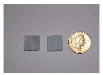
Fig. 6. HA / PLLA scaffolds as SLS produced
