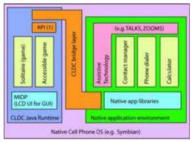
Fig. 27. CDC and CLDC with ÆGIS - accessibility API exposure to AT
