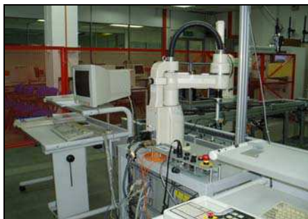
Fig. 12. The four degrees of freedom SCARA robot.
