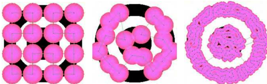
Fig. 11. ParaSOM in action: a) Hilbert initialized with a predetermined number of neurons; b) the network position at iteration 25; c) the network at iteration 500
