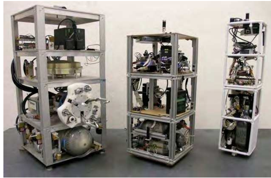
Fig. 1. Three generations of spacecraft simulator at the NPS Spacecraft Robotics Laboratory (first, second and third generations from left to right)
