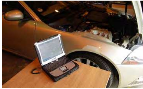
Fig. 9. Diagnostic tool for reading DTCs.
