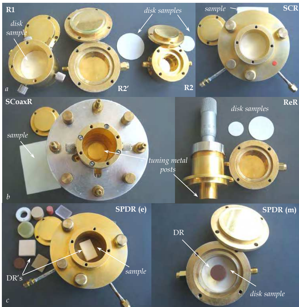
Fig. 6. Resonators' photos of different pairs: a) R1, R2, SCR; b) ReR; SCoaxR; c) SPDR's (e/m)
