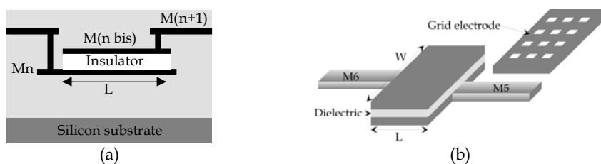
Fig. 2. Schematic view of a MIM capacitor: (a) cross-section, (b) 3D view
