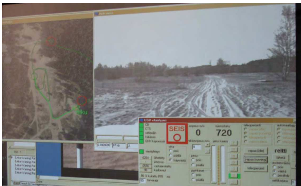
Fig. 6. User interface of the UGV demonstrator. On the left the map view of the demo area and on the right the video frame of the driving camera. Information about the vehicle state can be seen on the bottom right corner.
