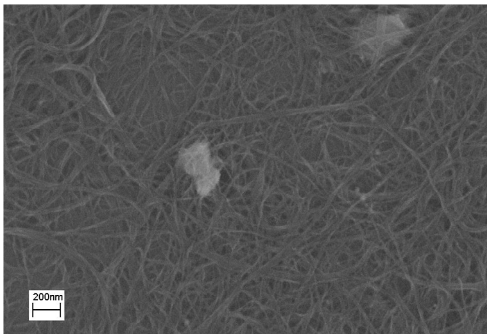
Fig. 1. SEM image of carbon nanotube arrays obtained by LB technique
