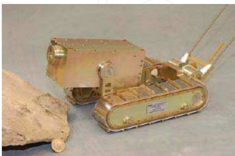
Fig. 6. Nanokhod dual-track system (Image Courtesy: Klinker, 2007)
