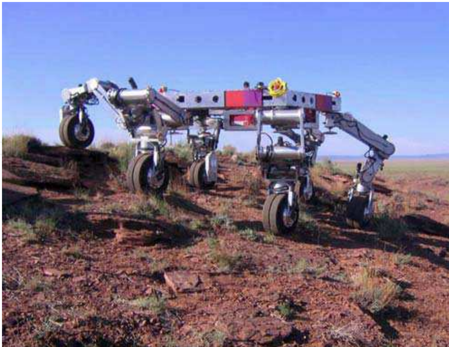
Fig. 14. Wheel-leg Hybrid system ATHLETE (Image Courtesy: NASA/JPL/Caltech)
