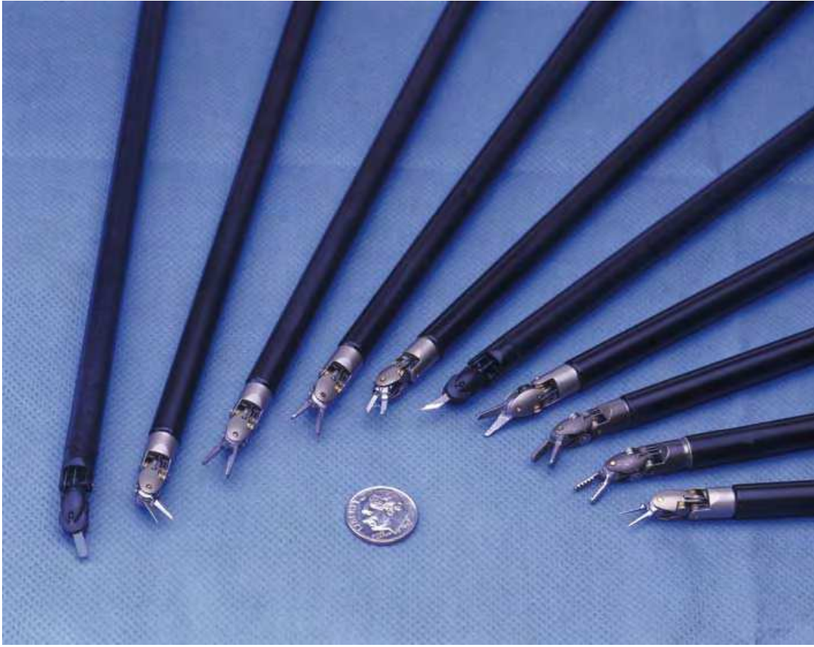
Figure 6. Range of available "wristed" instruments. EndoWrist ® ©[2007] Intuitive Surgical, Inc
