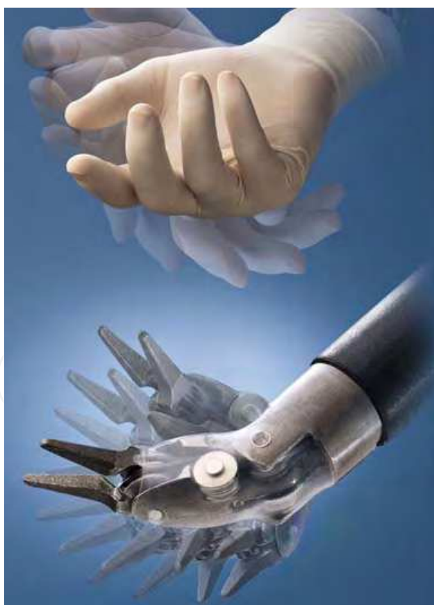
Figure 5. Demonstration of the 7 degrees of freedom with Endowrist® technology compared to surgeon hands. ©[2007] Intuitive Surgical, Inc
