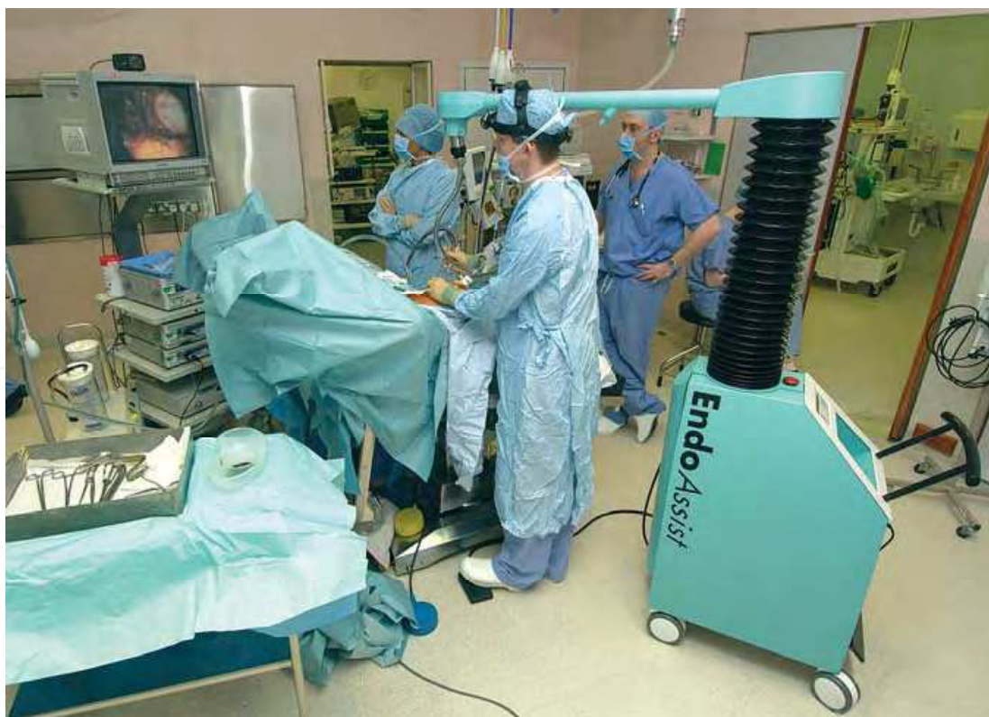
Figure 1. The EndoAssist manipulates a laparoscopic camera at the command of the surgeon. ©[2006] Prosurge, Limited
