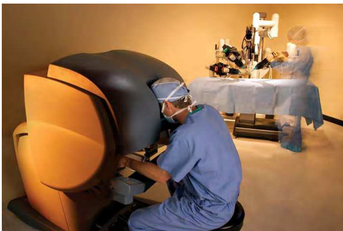
Figure 2. The da Vinci® robotic surgical system comprising of a surgeon's console and a patient side cart. ©[2007] Intuitive Surgical, Inc
