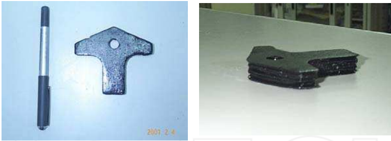
Fig. 20. RP part of Case 1 built by the proposed desktop manufacturing system
