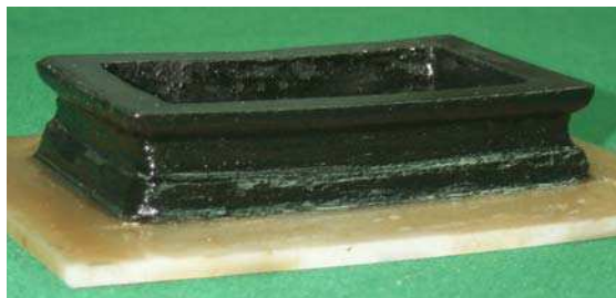
Fig. 23. RP part of Case 2 built by the proposed desktop manufacturing system The experimental results of Case 1 and Case 2 are also shown in Table 4.
