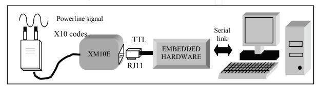
Fig. 10. Creating X10 applications with the XM10E module
