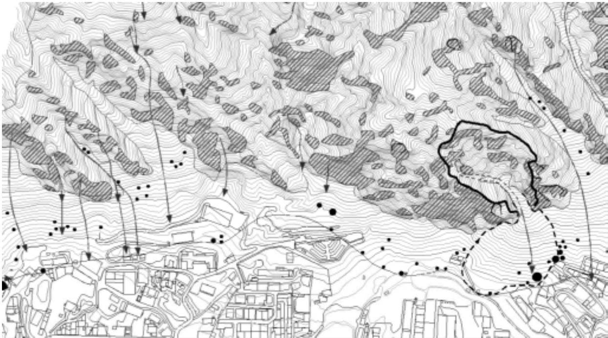
**Figure 6.** Boundary of the potential rockfall run-out area in Santa Coloma (Principality of Andorra), defined by the line that links the farthest fallen blocks observed in the field [24]. Arrows indicate historical rockfall paths and solid circles are large fallen boulders [65]
