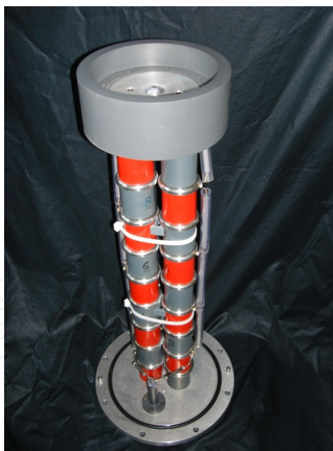
Figure 10. Photograph of the generator equipped with its load and referencing resistors
