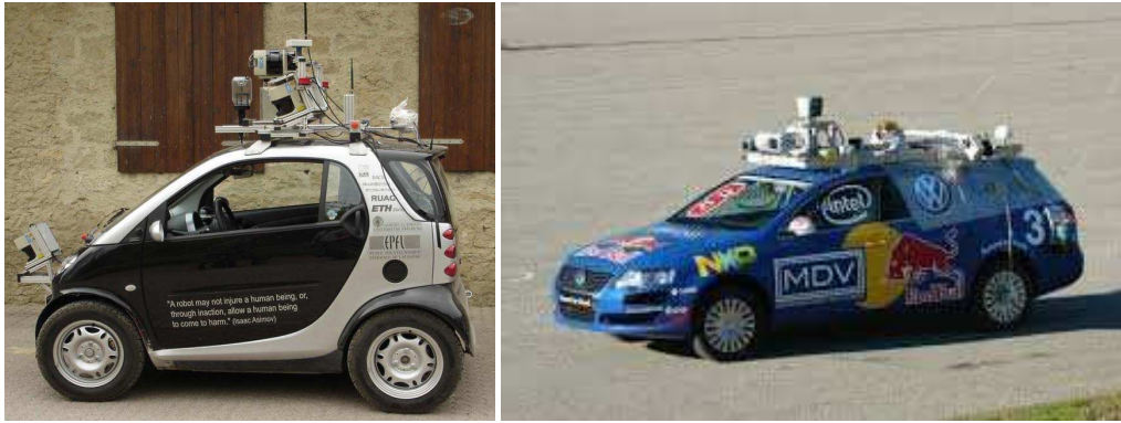
Figure 3. Two examples of autonomous self-driving car prototypes: the Smarter Car developed at ETH Zurich (left), and the Junior Car developed at Stanford University (right)
